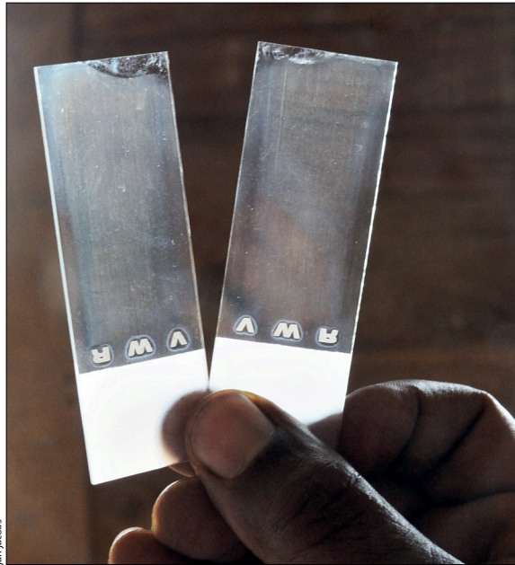
Figure 1: Adapted consumables for use in low-income settings At high relative humidity, glass slides for microscopy become opaque because of the development of condensation within the glass. Photograph taken in DR Congo.
